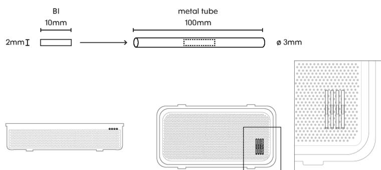
Figure 2: Scheme of the PCD and the most difficult site to sterilize in the container (top corner)
